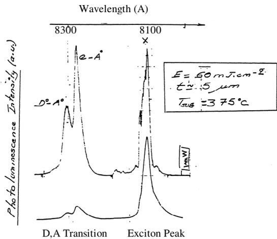
Fig 3. Undoped GaAs/GaAs MBE laser desorbed. Allows for low temperature growth
