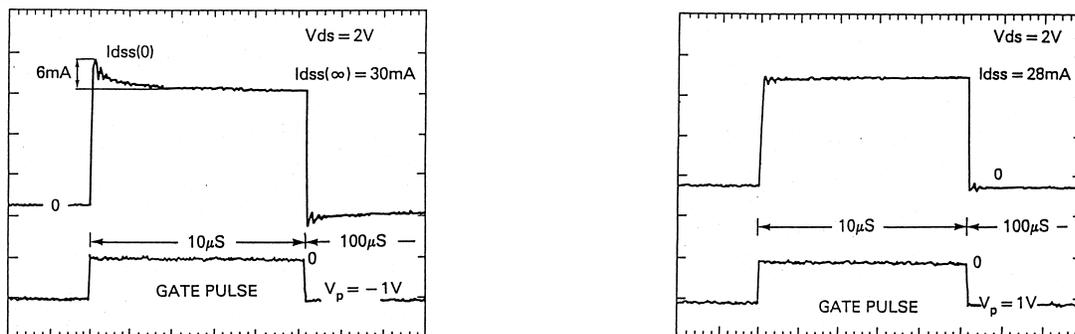
Fig 5 (a) Drain current response in normal HEFTs, and (b) Laser processed HEMTs
