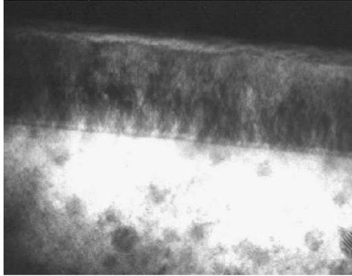
Figure 1. Transmission electron micrograph of GaAs/MgO/LSCO/PLZT/BST where the MgO layer is 25nm thick and the LSCO is 200nm thick.
