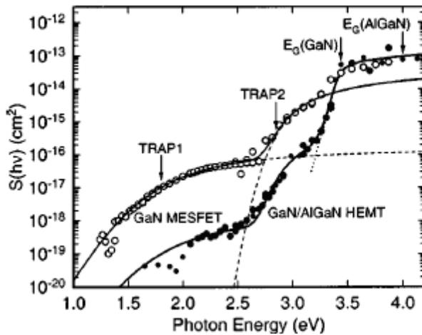
Figure 4. Photoionization spectra of a GaN MESFET and AlGaIn/GaN HEMT structure.
