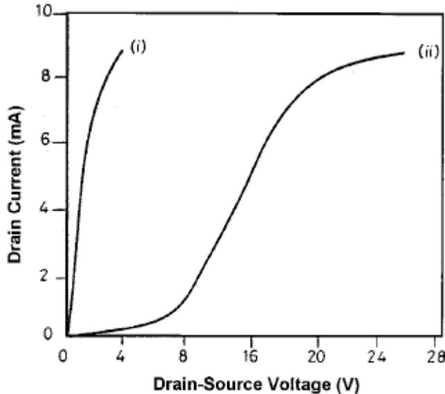
**Fig. 1.** Current collapse in an AlGaIn/GaN HEMT [32]. Drain current as a function of drain-source voltage (with the gate floating) is shown i) before and ii) after the application of a 20-V drain-source bias.
